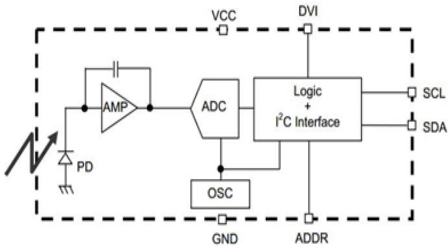
**Fig. 6.** BH1750FVI circuit diagram
