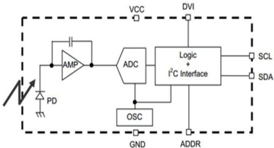
Fig. 6. BH1750FVI circuit diagram
