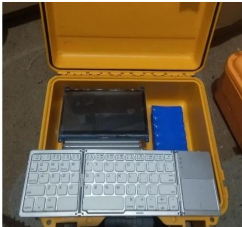
**Fig. 7.** Internal structure of the detection platform
