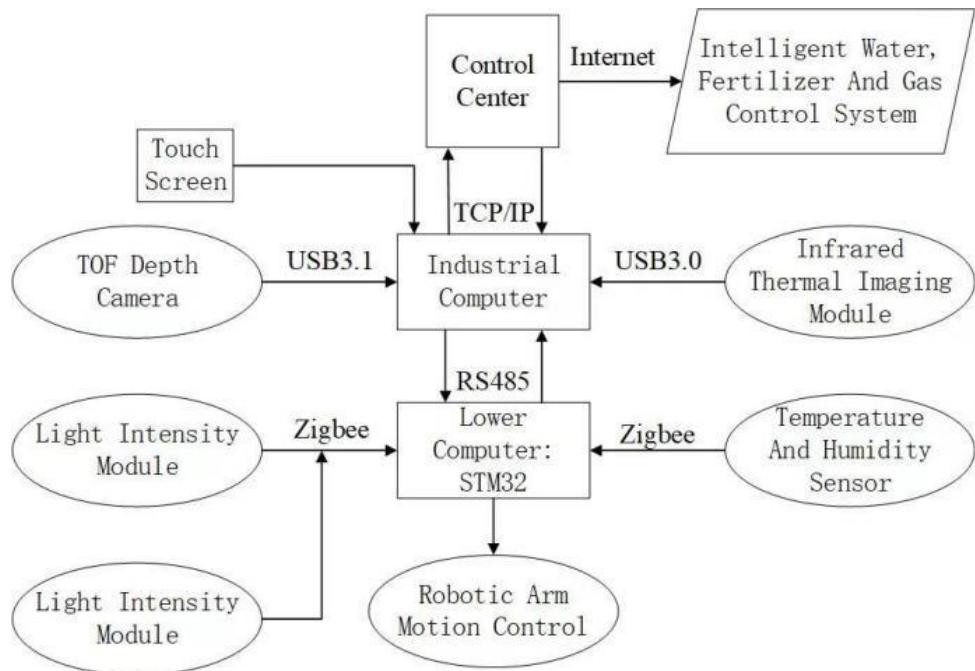
**Fig. 1.** Overall Scheme of Multi-source Sensor Integrated Detection Device
