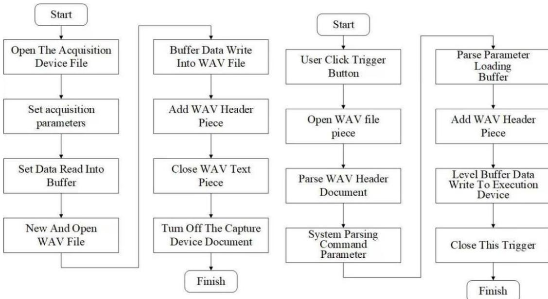
Fig. 10. Flowchart of software design of human-computer interaction interface
