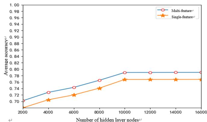
Fig.6 Accuracy of Different Number of Hidden Nodes
