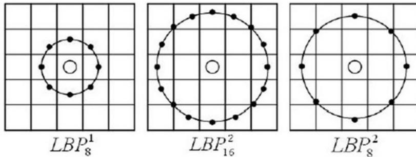
Fig.1 Circular LBP operator with radius of  $R$  containing  $P$  sampling points
