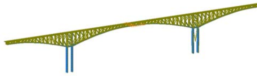
Fig.5. Mode of truss members instability on the top of pier
