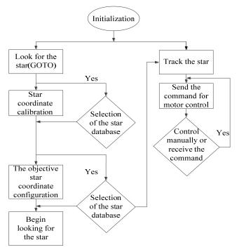
Fig. 3 Telescope Control Program Flow Chat
