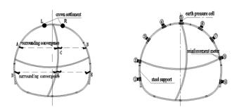
(a) crown settlement and surrounding convergence (b) surrounding rock pressure and steel bracing force Fig. 2 Measuring points arrangement
