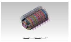
(a) Coupling Mesh of tunnel(b) Initial and temporary support structureFig.7 FEM model of the tunnel and its supporting structure
