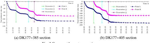
Fig. 3 Crown settlement versus time curves
