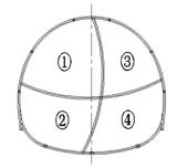
Fig. 1 Excavation sequence of Liangcun tunnel
