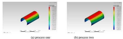
Fig.9 Stress contour of sprayed concrete in two processes
