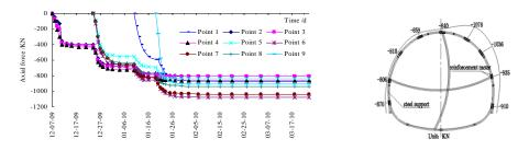
(a) Axial force of steel support versus time curves(b) Axial force of steel support distributionFig.6 Axial force of steel support and its time-history curves at DK177+385 section
