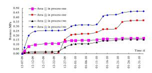
Fig.10 Surrounding rock pressure versus time curves
